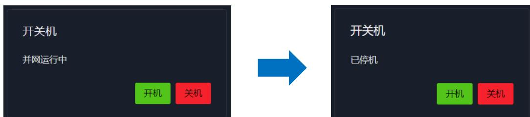
**Step 4** Check the "Home" screen to verify that the PCS is in inactive mode, indicating that the equipment has been shut down.
